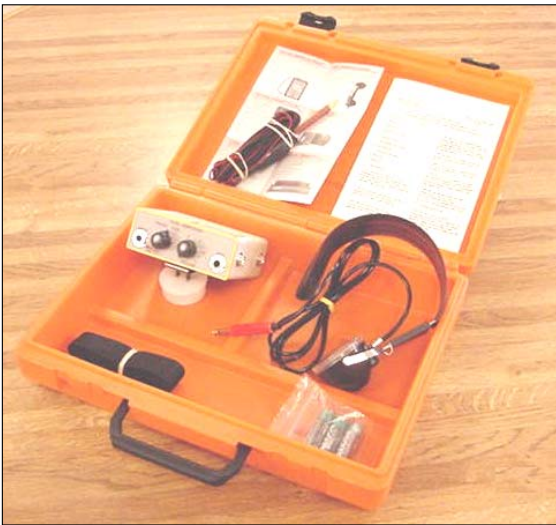
FIG. 1 MT-91A TEST SET INCLUDES: MT-147D AMPLIFIER (PN: 86-100-017) MT-513A PROBE (P/N: 86-100-059) MT-723A HEADSET (P/N: 86-100-005) CARRYING STRAP (P/N: 82-48-069)
